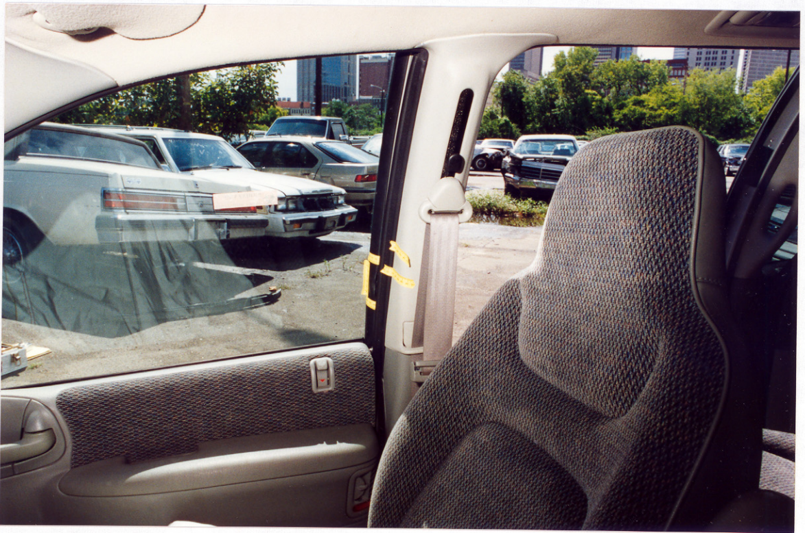
93. View of a rebound contact at the right B-pillar/window juncture.
